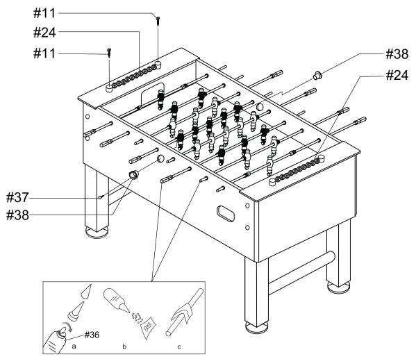
Spray the lubricant into a clean, soft cloth and then use the cloth to wipe the player rods where they come into contact with the bearings. See pictured above.
